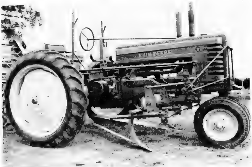
Figure 7.—Tractor with digger blades.
