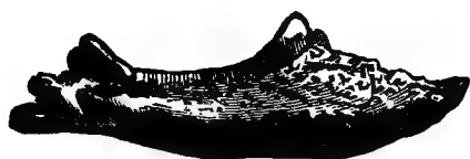
FIG. 779.—Side View of the Above, Showing Bending up of the Edges, etc.
