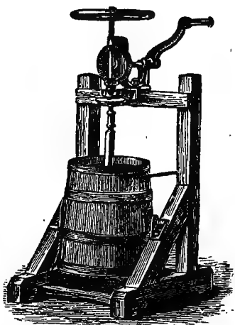
FIG. 879.—Small Holstein Vertical Churn.
