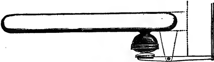
FIG. 1873.—Regulator of Tomlinson's Incubator.
