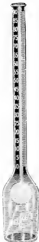
FIG. 27.—Illinois 9 inch, 9 gram, 90 per cent butter test bottle.
