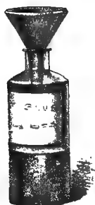
FIG. 12.—Small narrow-mouthed bottle fitted with funnel filter, used especially for aniline staining fluids and aniline water.
