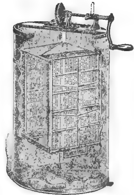
Fig. 20.—Honey extractor, used to remove honey from the combs without destroying them
