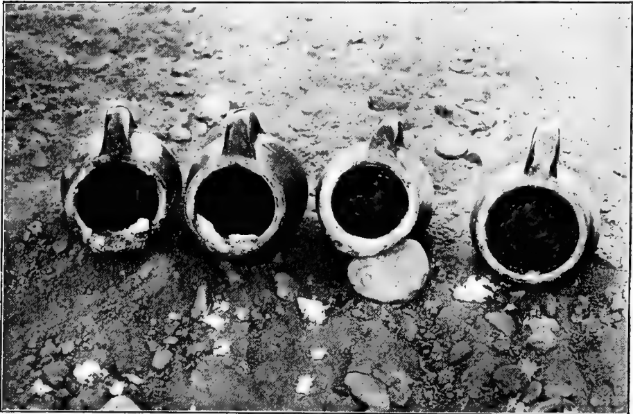
FIG. 52.—Acid generators showing residue remaining because of careless emptying. (After Pierce, P. C. Jr. Ent.)
