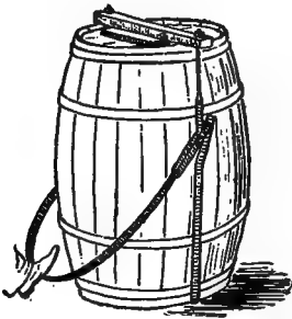
FIG. 16—ORDINARY LEVER PRESS FOR APPLE BARREL
