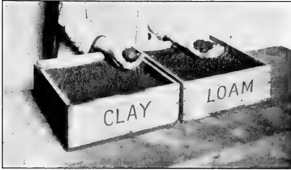
FIG. 39. The clay soil is easily made into a ball, while the loam falls apart. This shows that the loam is in good condition for working, and that the clay is too wet.
