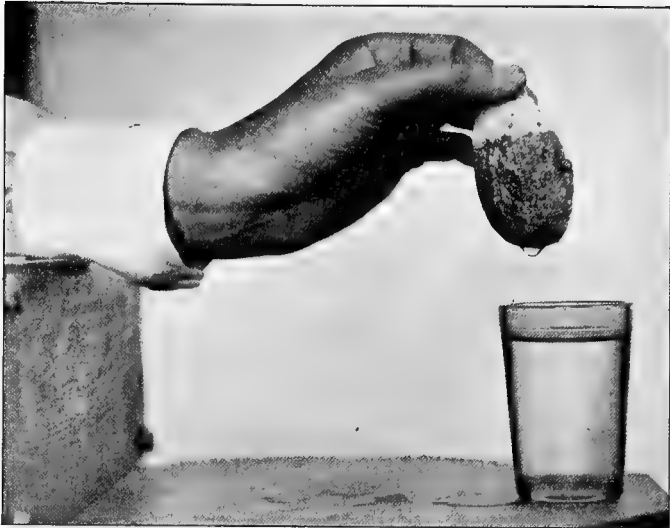
FIG. 48. On the surface of the stone is a thin film of capillary water; at the bottom is a drop of free water.
