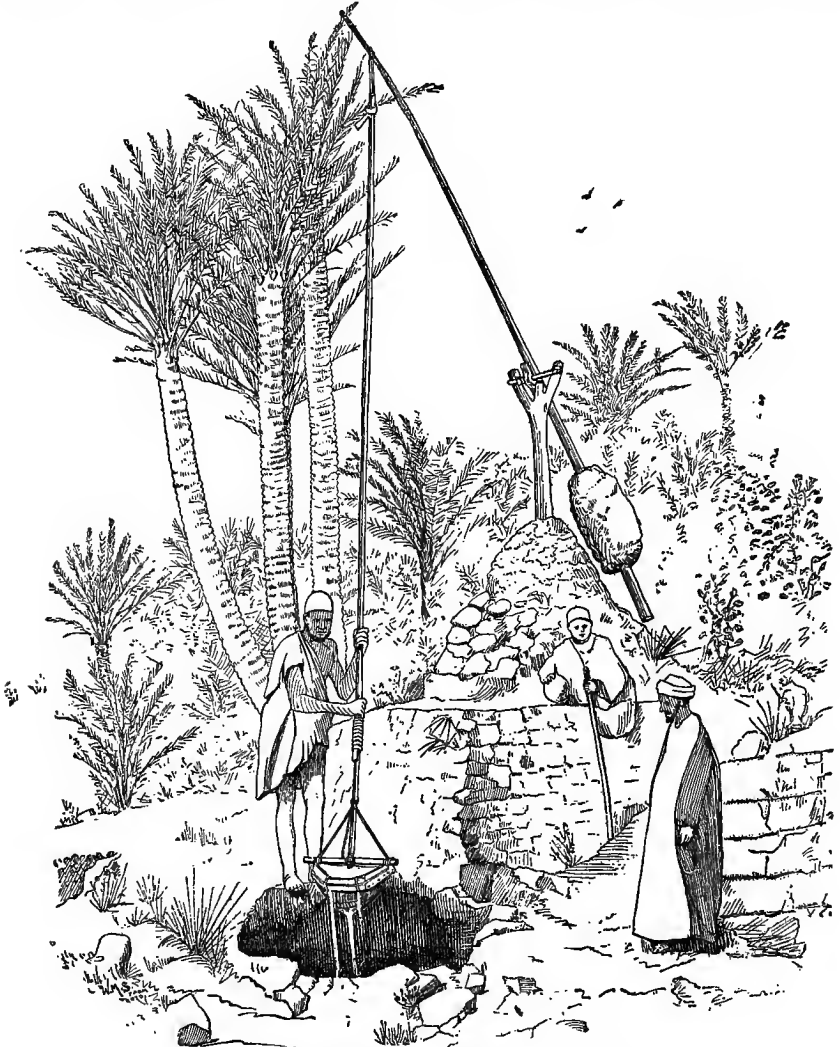
FIG. 1.—Raising water from well in India by paecottah.
