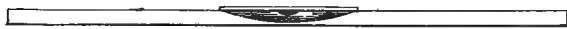
Longitudinal section of hollow-ground glass slide for observing bacteria in hanging drops.
