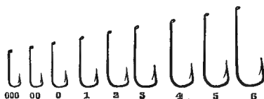
OLD PATTERN OF TURN-DOWN EYED 'PENNELL-SNECK' HOOKS. (Patent U.S.A.)
