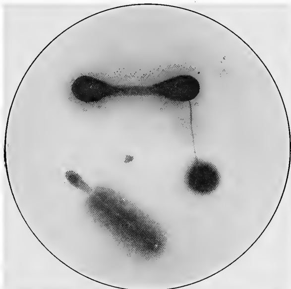
FIG. 23. — A piece of mill scale is shown in the center. Shows the stimulated corrosion of iron affected by contact with the electro-negative magnetic oxide of iron. (Walker.)
