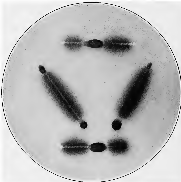
FIG. 12.—Steel nails in ferroxyl reagent. (Walker.)
