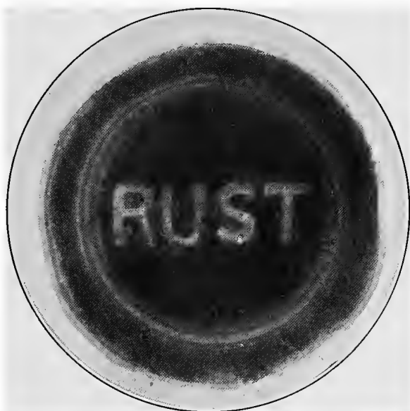
FIG. 31. — Showing the effect produced in the ferroxyl indicator by cutting the surface of a polished steel plate. (Cushman.)
