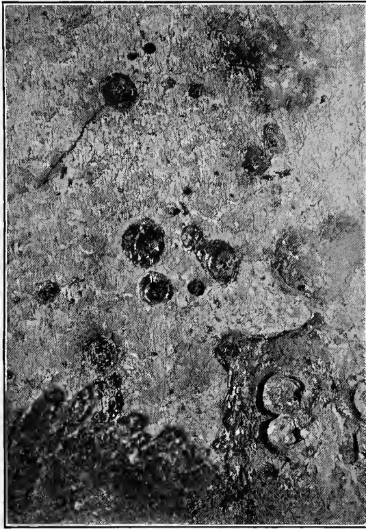
FIG. 17. — Photographic representation of rust-spots formed on the surface of iron.
