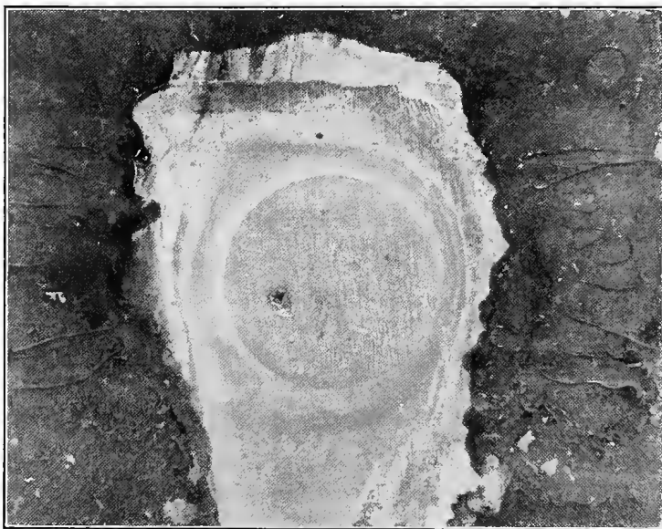
FIG. 32. — Illustrating the protection on the surface of the steel in the immediate neighborhood of a button of zinc soldered into the steel. The sphere of influence of the zinc is shown to be proscribed. (Cushman.)
