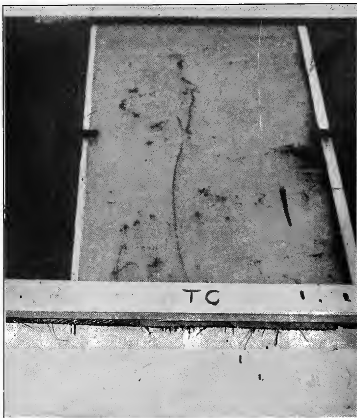
FIG. 37. — Charcoal iron tinned plate, showing the corrosion lines.
