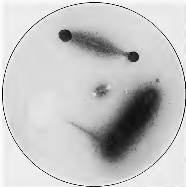
FIG. 22. — A piece of zinc is shown in the center. Shows the protective action of the electro-positive metal, zinc, on the corrosion of iron. (Walker.)
