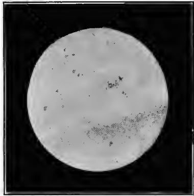
FIG. 43 (c). — Paint coating composed of zinc oxide, lead sulphate, and silica, showing no salt crystals.
