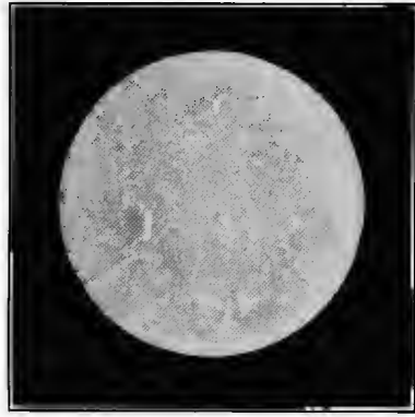
FIG. 43 (b). — Fine crystals of salt on asbestine panel.
