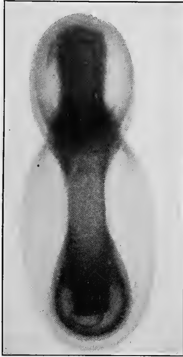
FIG. 13. — Strip of steel in ferroxyl reagent, showing frequent shifting of poles. (Cushman.)
