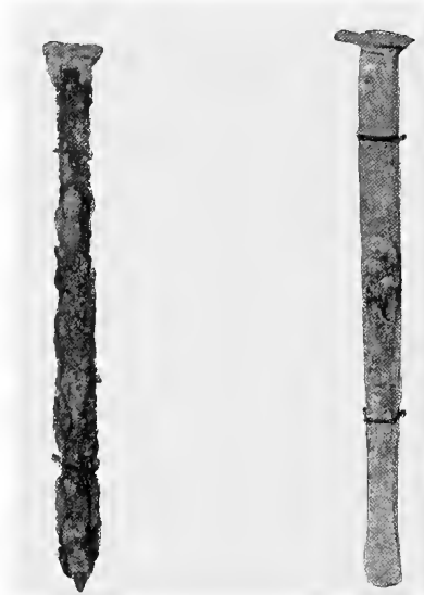
FIG 1. — Showing the relative corrosion of a modern steel nail and an old forged nail.
