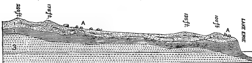
1. Sand, gravel, and clay. 2. Erie clay, laminated. 3. Erie shale. A A. Bowlders.
