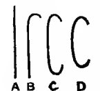
Fig. 139.—Different stages of bending the Centre-bouts.
