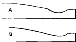
FIG. 148.—Stages of the cutting in sinking the edges.
