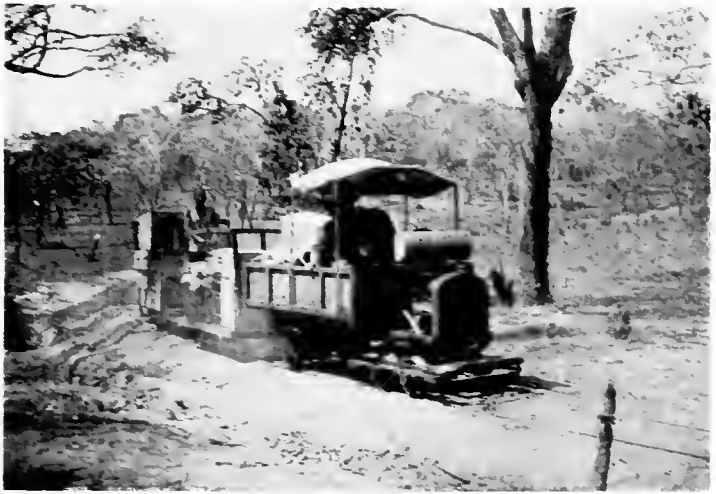
THE LIGHT RAILWAY IN THE LINDI AREA ANOTHER USE FOR THE FORD CAR
