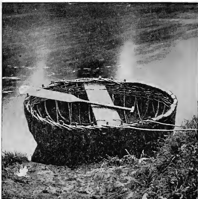
Fig. 216.— Currach or coracle used on the Boyne, Ireland. (From photograph by R. Welch.)
