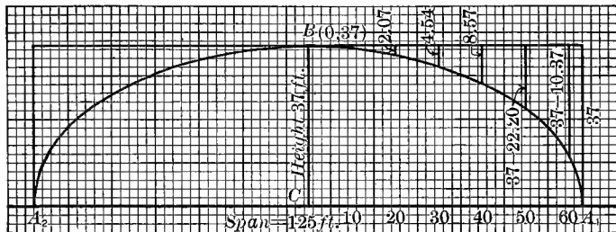
Elliptical arch, 125 foot span by 37 feet high
