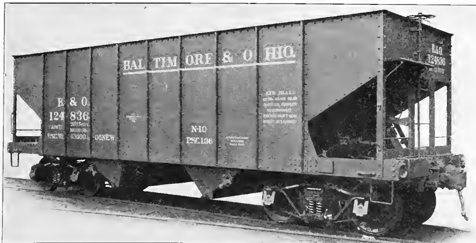
Fig. 70. Steel Hopper Car. Capacity, 100,000 lbs. Weight, 43,600 lbs. Pressed Steel Car Co., Builders. (Drawings of this car are shown in Figs. 490-495.)
