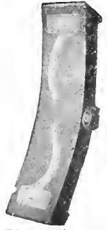
Fig. 5238. Streeter Shoe with White Iron Inserts.
