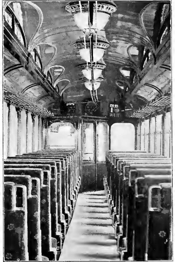
Fig. 6247. Interior of High Speed Interurban Car. Canton-Akron Ry. St. Louis Car Co., Builders.
