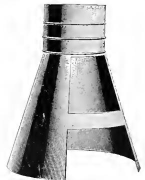
Fig. 2695. Base of Smoke Flue.
