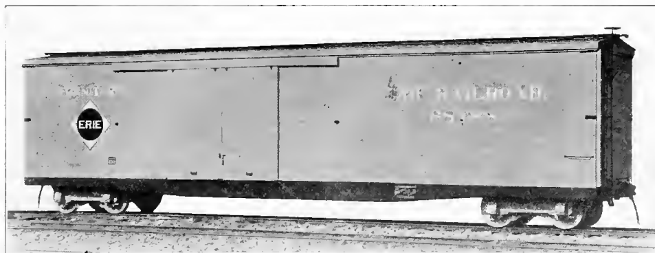
Fig. 3. Furniture Car, Pressed Steel Underframe. Capacity, 60,000 lbs. Weight, 44,000 lbs. Length, 50 ft. Pressed Steel Car Co., Builders. (Drawings of this car are shown in Figs. 287-290.)
