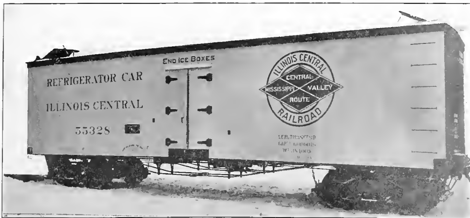
Fig. 16. Refrigerator Car with End Ice Boxes. Capacity, 60,000 lbs. Weight, 38,400 lbs. Length, 38 ft., 8 in. American Car & Foundry Co., Builders. (Drawings of this car are shown in Figs. 305-308.)
