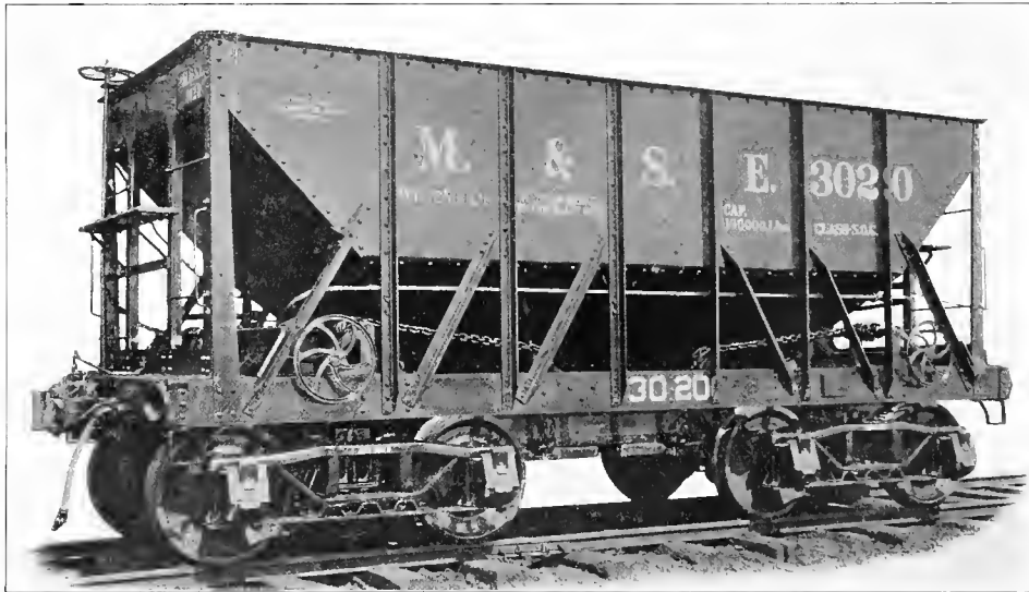
Fig. 72. Ore Car, Pressed Steel. Capacity, 100,000 lbs. Weight, 32,800 lbs. Pressed Steel Car Co., Builders.
