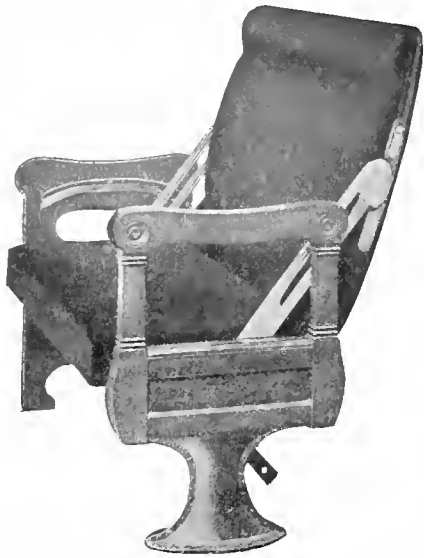
Fig. 4107. Reversible Seat, No. 179. Plush Upholstery. N. Y., N. H. & H. Type for Vestibuled Coaches.
