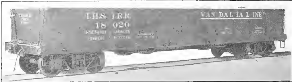
Fig. 40. Gondola Car, Drop Bottom and Ends, Pressed Steel. Capacity, 100,000 lbs. Weight, 39,900 lbs. Pressed Steel Car Co., Builders.
