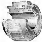
Fig. 6345. Commutator Construction, G.E.-216 Railway Motor.
