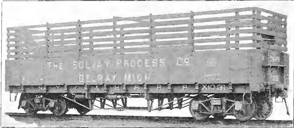
Fig. 56. Gondola Car with High Coke Racks. Capacity, 80,000 lbs. Middletown Car Co., Builders. (Drawings of this car are shown in Figs. 381-382.)
