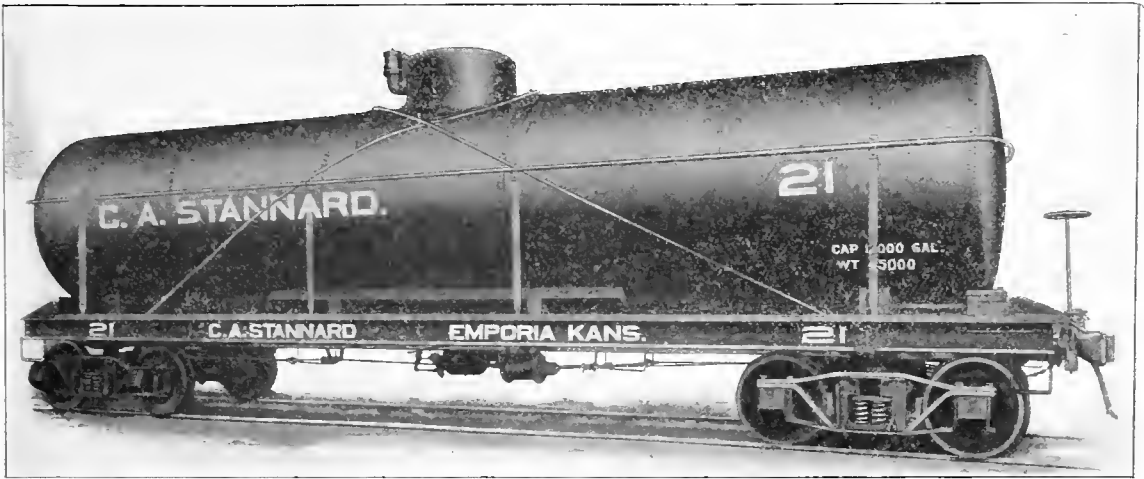
Fig. 125. Tank Car, Structural Steel Underframe. Capacity, 12,000 gals. Weight, 45,000 lbs. McGuire-Cummings Mfg. Co., Builders.
