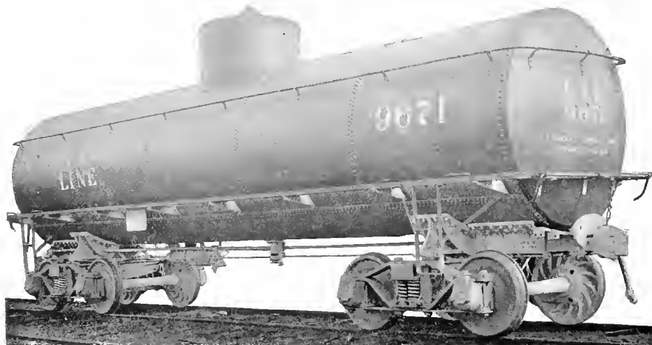
Fig. 128. Tank Car, Van Dyke Patent. Capacity, 10,000 gals. (Drawings of this car are shown in Figs. 554-558.)
