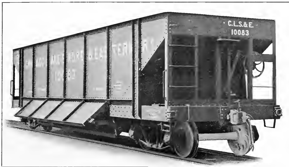
Fig. 76. Coke Car. All Steel, Self Clearing. Capacity, 100,000 lbs. Weight, 47,600 lbs. American Car & Foundry Co., Builders.
