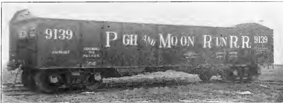
Fig. 46. Gondola Car, Drop Bottom, High Side. Capacity, 90,000 lbs. Weight, 37,200 lbs. American Car & Foundry Co., Builders.
