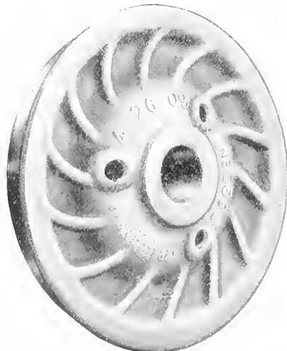
Figs. 5464-5465. 33-Inch, 665-lb. Double Plate Cast Iron Wheel for 80,000 lbs. Capacity Freight Cars, Griffin Wheel Co.
