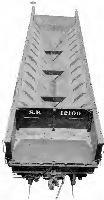
Fig. 89. Hart Convertible Car Arranged for Center Dumping Ballast.
