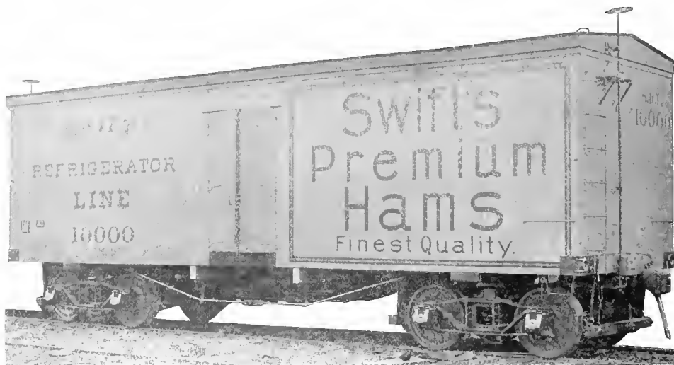
Fig. 17. Refrigerator Car, Wooden Underframe, Bowen Patent. Capacity, 50,000 lbs. Weight, 35,800 lbs. American Car & Foundry Co., Builders.
