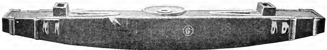
Fig. 5046. V-Shape Cast Steel Truck Bolster. American Steel Foundries.
