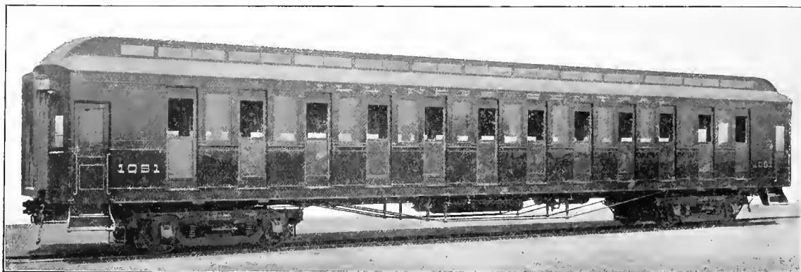
Fig. 202. Side-Door Suburban Car with Steel Underframe. Illinois Central. (Drawings of this car are shown in Figs. 650-634.)
