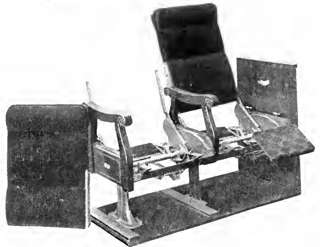
Fig. 4137. Mechanism of Double Reclining Chair Seat Barney & Smith Car Co.
