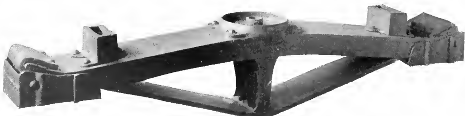
Fig. 5048. Simplex Truck Bolster for 80,000 lbs. Capacity Car. Simplex Railway Appliance Co.
