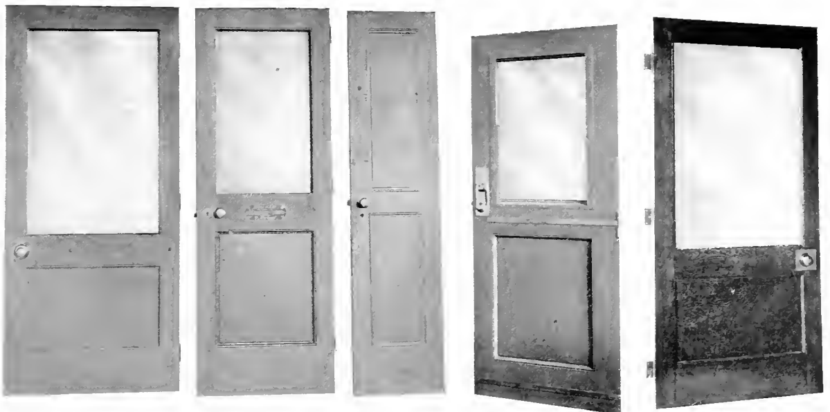
Fig. 1343. Steel Vestibule Door. Exterior. Fig. 1344. Steel End Door. Exterior. Fig. 1345. Steel Saloon Door. Exterior. Fig. 1346. Steel End Door. Hudson & Manhattan Steel Tunnel Car Doors. Fig. 1347. Steel End Door. Harriman Lines Standard Steel Coach Door.
