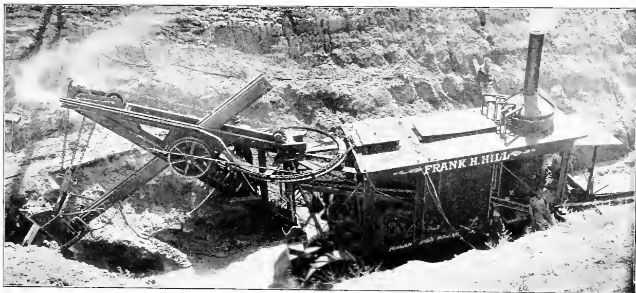
Fig. 254. 32-Ton "Little Giant" Traction Wheel Shovel. The Vulcan Steam Shovel Co., Builders.
