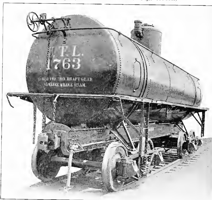
Fig. 129. Tank Car, Structural Steel Underframe. Capacity, 6,000 gals. (Drawings of this car are shown in Figs. 559-561.)
