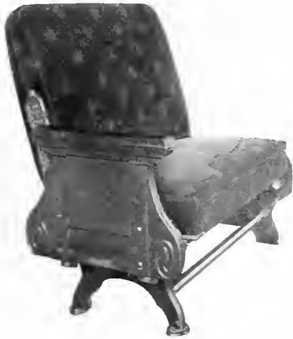
Fig. 4101. Steel Walkover Seat, No. 194. Frieze Plush Upholstery. P. R. R. Standard for Steel Coaches.
