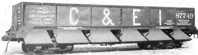
Fig. 87. Dump Car, Steel Side and Underframe. Capacity, 100,000 lbs. Weight, 38,900 lbs. Length, 36 ft., 6 in. National Dump Car Co., Builders.
