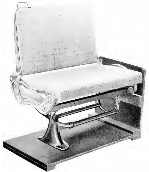
Fig. 6418. "Winner" Pushover Back Seat, with Cast or Pressed Steel Pedestal.
