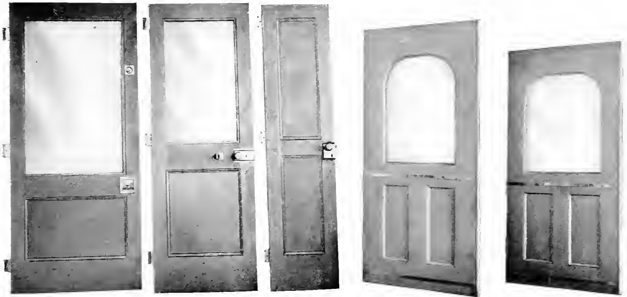
Fig. 1338. Steel Vestibule Door. Interior. Fig. 1339. Steel End Door. Interior. Fig. 1340. Steel Saloon Door. Interior. Figs. 1341-1342. Steel Sliding Doors. Hudson & Manhattan Steel Tunnel Car Doors. P. R. R. Standard Steel Coach Doors.
