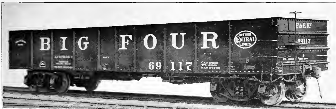
Fig. 35. Gondola Car, Twin Hopper, All Steel. Capacity, 100,000 lbs. Weight, 42,600 lbs. Length, 40 ft. Barney & Smith Car Co., Builders.
