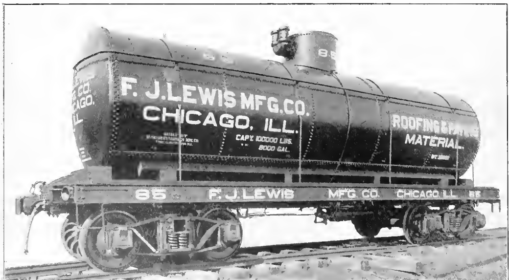
Fig. 124. Tank Car, Structural Steel Underframe. Capacity, 8,000 gals. Weight, 38,000 lbs. McGuire-Cummings Mfg. Co., Builders. (Drawings of this car shown in Figs. 569-671.)
