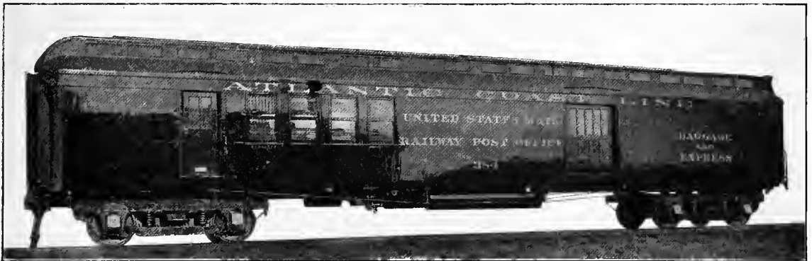
Fig. 200. Combination Postal and Baggage Car. Atlantic Coast Line. Hicks Locomotive & Car Works, Builders.
