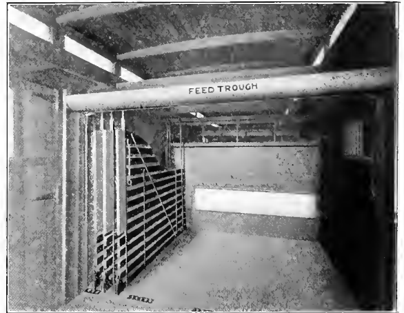
Fig. 116. Interior of "Perfected" Horse Car Showing Stall Partitions Shifted to One Side.
