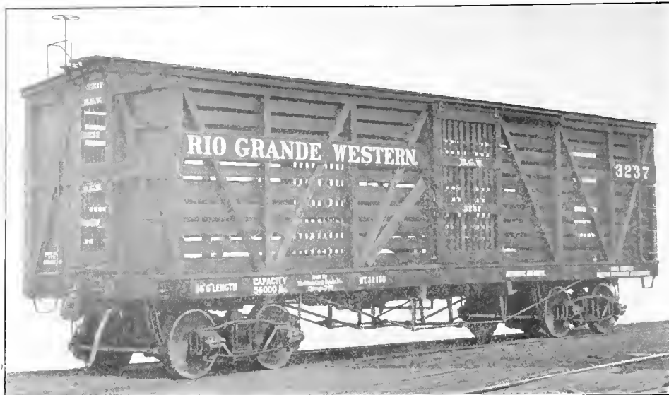
Fig. 108. Stock Car. Capacity, 56,000 lbs. Weight, 32,100 lbs. Length, 36 ft., 6 in. Western Steel Car & Foundry Co., Builders.
