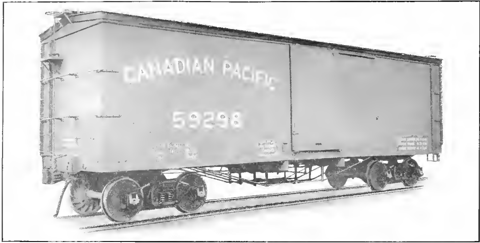
Fig. 11. Box Car, Wooden Underframe. Capacity, 60,000 lbs. Weight, 36,200 lbs. Length, 36 ft. American Car & Foundry Co., Builders.
