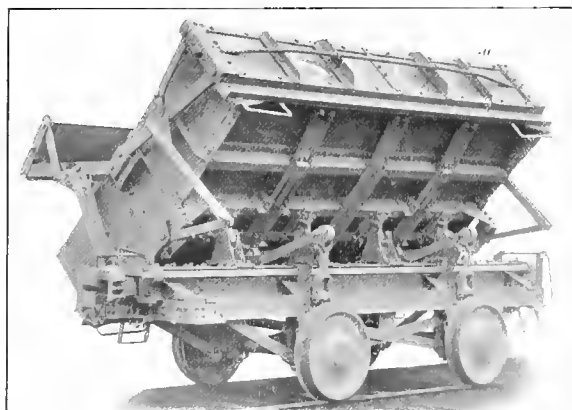
Figs. 99-99a. Seven-Yard Double Dump Car. Russel Wheel & Foundry Co., Builders.
