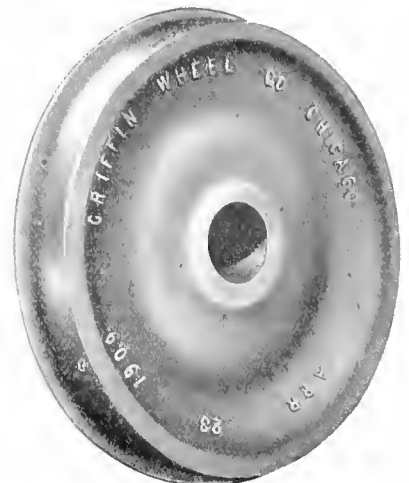
Figs. 5464-5465. 33-Inch, 665-lb. Double Plate Cast Iron Wheel for 80,000 lbs. Capacity Freight Cars, Griffin Wheel Co.
