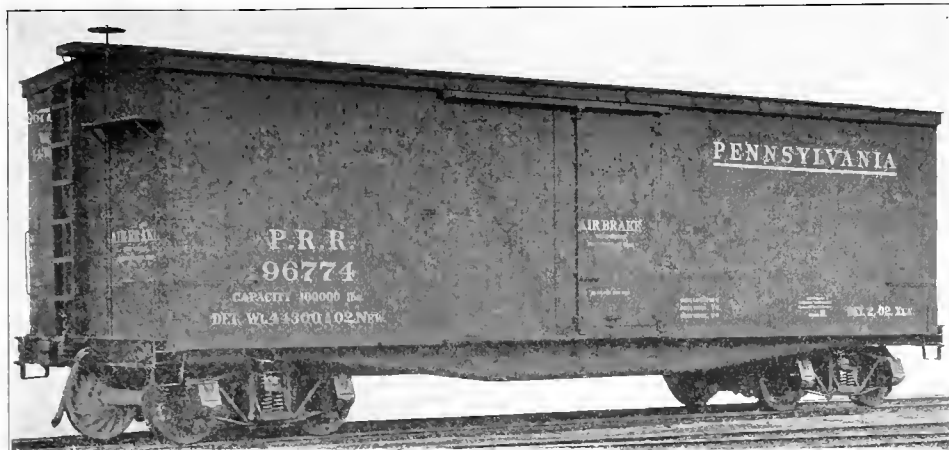
Fig. 1. Box Car, Pressed Steel Underframe. Capacity, 100,000 lbs. Weight, 44,300 lbs. Length, 36 ft. American Car & Foundry Co., Builders. (Drawings of this car are shown in Figs. 266-268.)
