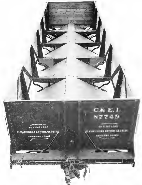
Fig. 86. National Dump Car with Drop Doors Open.
