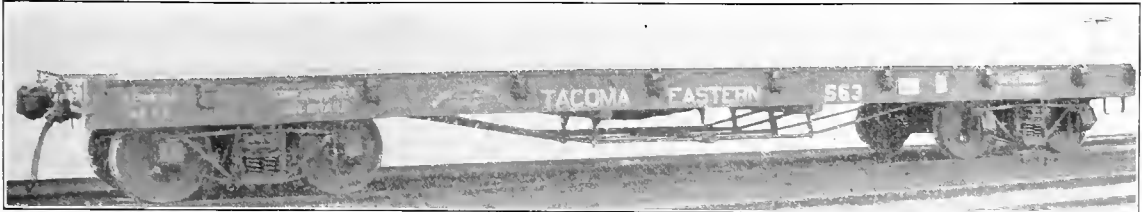
Fig. 26. Flat Car, Wooden Underframe. Capacity, 80,000 lbs. Weight, 27,200 lbs. Length, 41 ft. American Car & Foundry Co., Builders.
