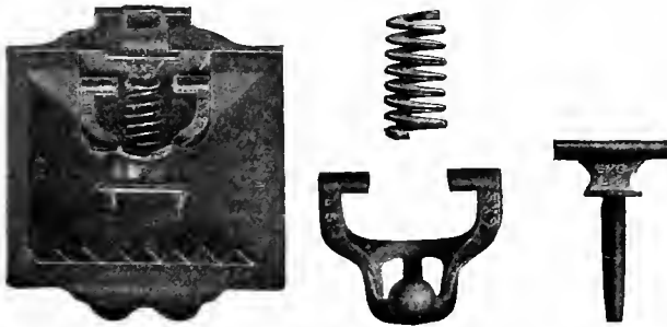
Figs. 5272-5275. Climax Journal Box Lid and Parts in Detail.
