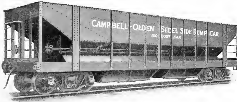
Fig. 95. Campbell-Olden Steel Side Dump Car. Capacity 100,000 lbs. Joliet Steel Car Mfg. Co., Builders. (Drawings of this car are shown in Figs. 543-544.)
