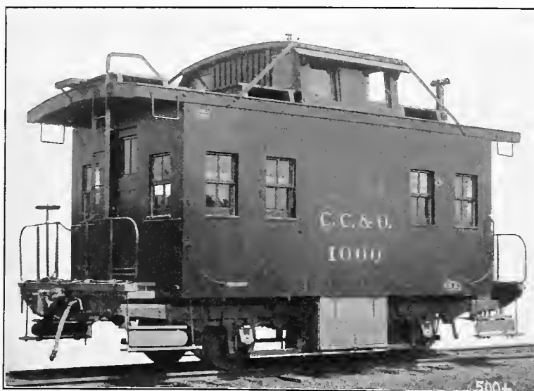
Fig. 121. Caboose Car, Steel Underframe. Hicks Locomotive & Car Works, Builders.
