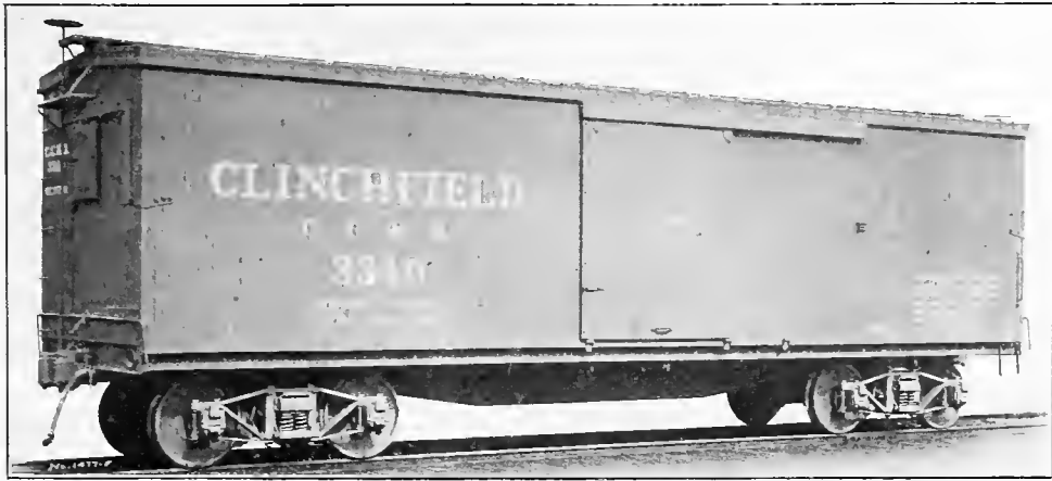
Fig. 8. Box Car, Structural Steel Underframe. Capacity, 60,000 lbs. Weight 35,700 lbs. Length 36 ft. Pressed Steel Car Co., Builders.
