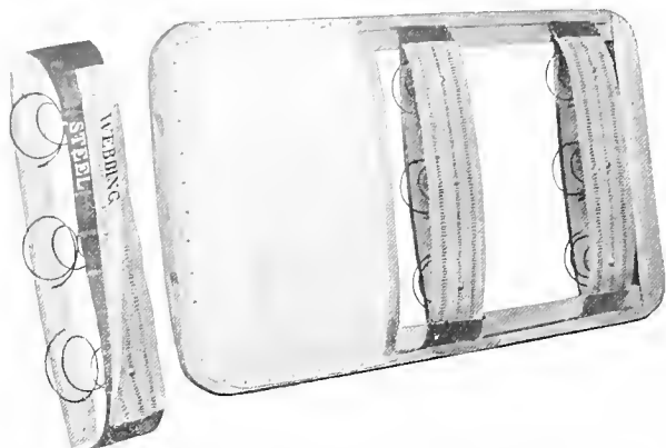
Figs. 4166-4167. Improved Combination Spring Back. One Section is Detached.
