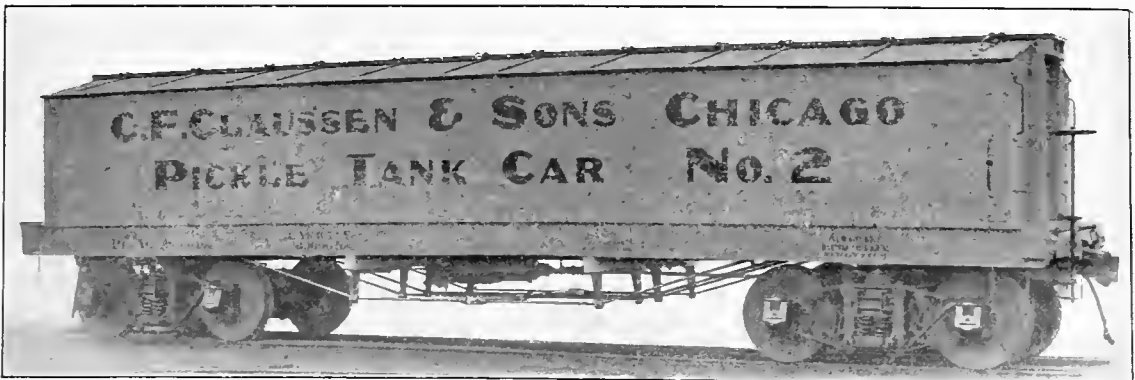
Fig. 127. Pickle Tank Car, Three Compartments. Capacity, 60,000 lbs. Weight, 37,300 lbs. Middletown Car Co., Builders.
