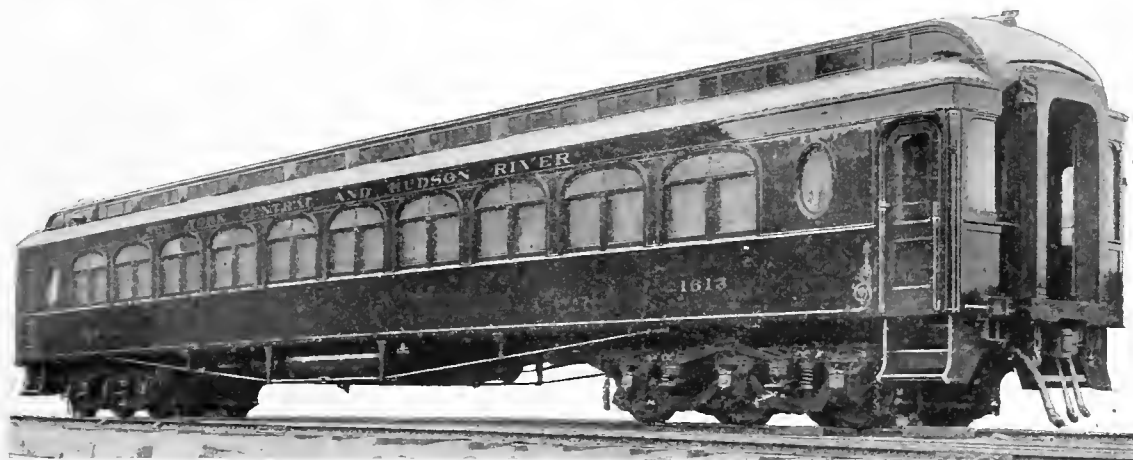
Fig. 135. Standard Coach, New York Central. Barney & Smith Car Co., Builders. (Floor plan of this car is shown in Fig. 227.)
