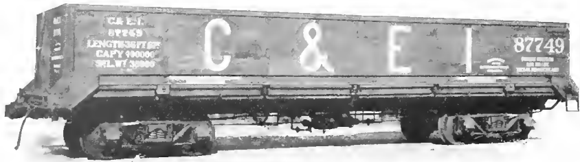
Fig. 84. Dump Car, Steel Sides and Underframe. Capacity, 100,000 lbs. Weight, 38,900 lbs. Length, 36 ft., 6 in. National Dump Car Co., Builders.
