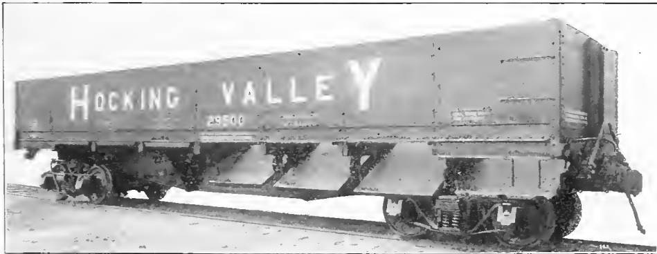
Fig. 81. Dump Car, Drop Bottom, Flush Floor, Steel Underframe. Capacity, 100,000 lbs. Weight, 41,000 lbs. Ralston Steel Car Co., Builders.
