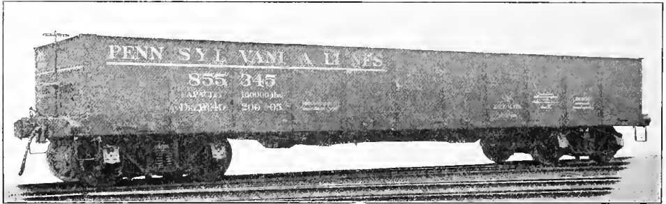
Fig. 49. Gondola Car, Drop Bottom, Pressed Steel. Capacity, 100,000 lbs. Weight, 40,200 lbs. Length, 38 ft., 2½ in. American Car & Foundry Co., Builders.
