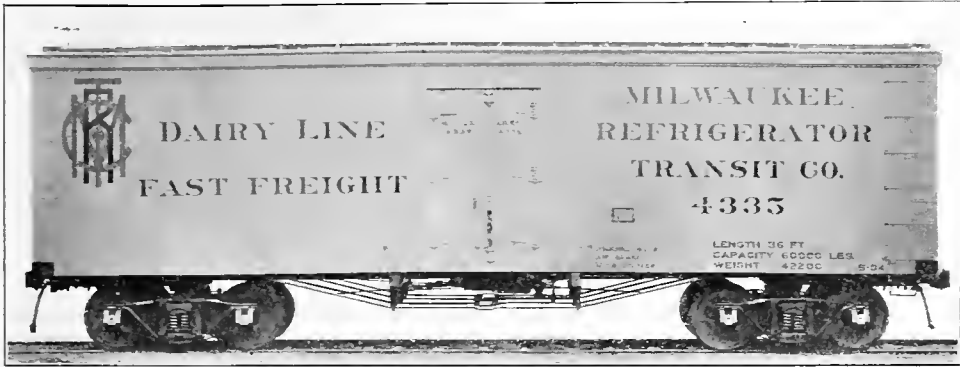
Fig. 20. Refrigerator Car for Dairy Products. Capacity, 60,000 lbs. Weight, 42,200 lbs. Length, 36 ft. Milwaukee Car Mfg. Co., Builders.
