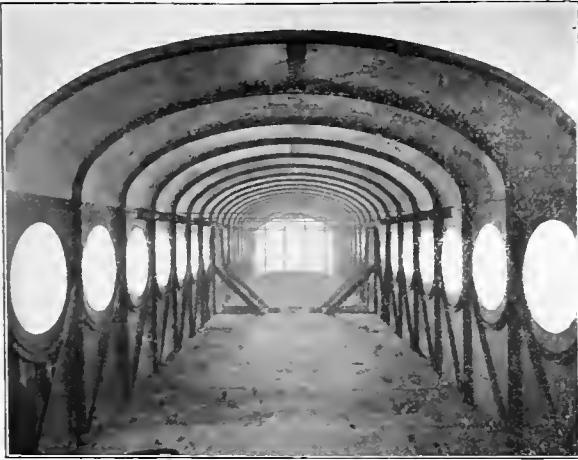
Figs. 1040-1041. Interior Views of Partially Completed All Steel Union Pacific Passenger Coach, No. 499. (Exterior view of this car shown in Fig. 140.)
