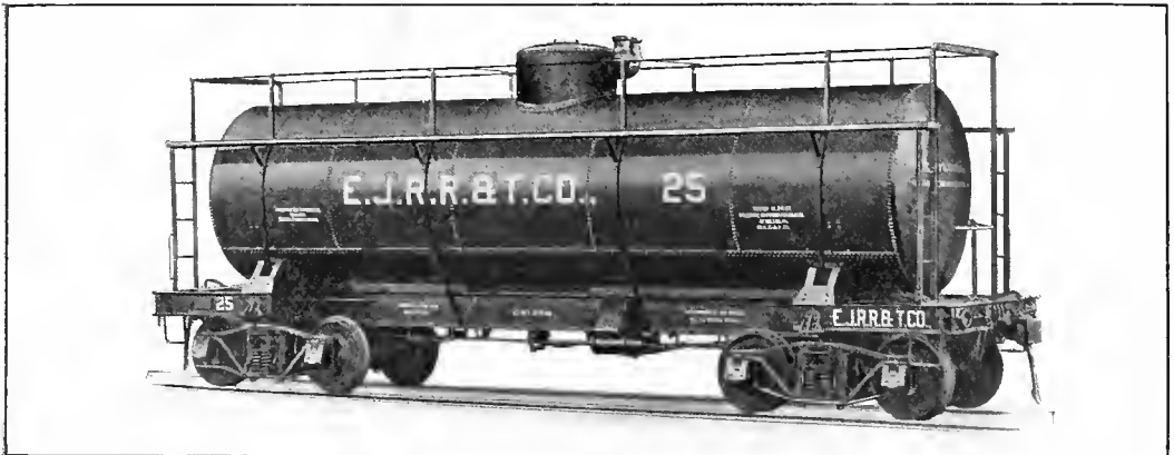
Fig. 123. Tank Car, Structural Steel Underframe. Capacity, 12,850 gals. American Car & Foundry Co., Builders. (Underframe of this car shown in Fig. 1030.)
