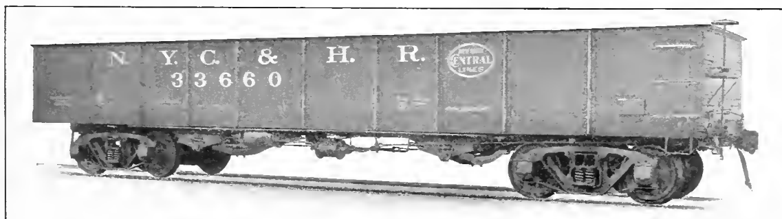
Fig. 36. Gondola Car, Twin Hopper, All Steel. Capacity, 100,000 lbs. Weight, 38,800 lbs. Length, 40 ft. American Car & Foundry Co., Builders.
