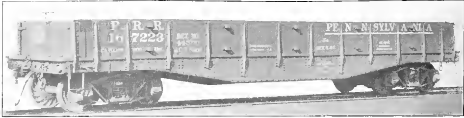
Fig. 39. Gondola Car, Drop Ends, Wooden Body, Pressed Steel Underframe. Capacity, 100,000 lbs. Weight, 14,500 lbs. Pressed Steel Car Co., Builders. (Drawings of this car are shown in Figs. 388-391.)
