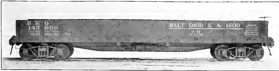
Fig. 44. Gondola Car, Flat Bottom, Structural Steel Underframe, Wooden Body. Capacity, 100,000 lbs. Weight 44,800 lbs. Standard Steel Car Co., Builders. (Drawings of this car are shown in Figs. 411-413.)
