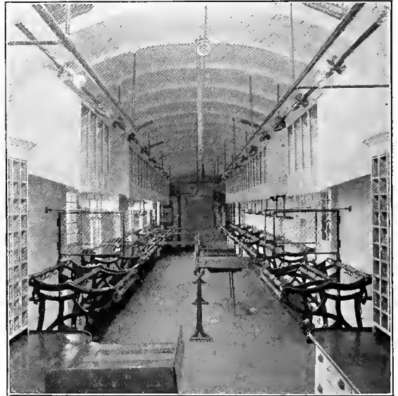
Fig. 196. Interior of All Steel Postal Car. U. P. Union Pacific Railroad Co., Builders.
