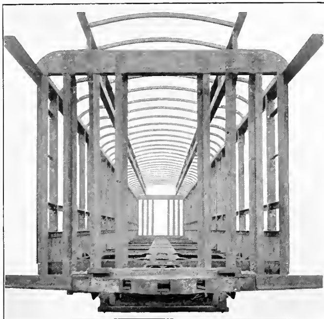
Fig. 1043. Steel Framing of C., M. & St. P. Library Buffet Car "Winneconne."
