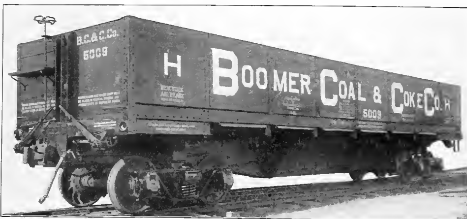
Fig. 83. Dump Car, Drop Bottom, Flush Floor, Steel Underframe. Capacity, 100,000 lbs. Weight, 41,000 lbs. Ralston Steel Car Co., Builders.
