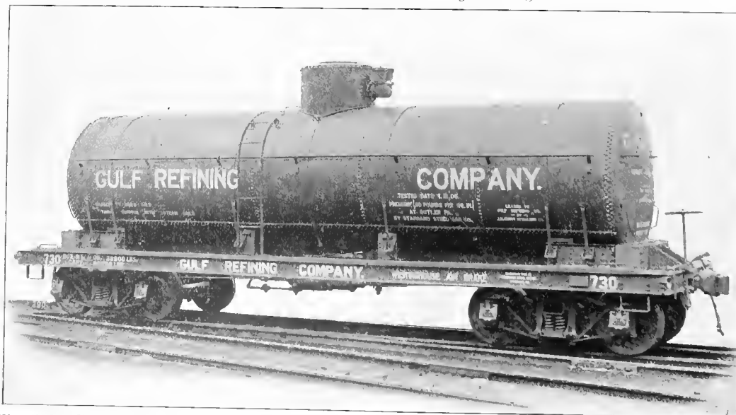
Fig. 130. Tank Car, Structural Underframe. Capacity, 8,020 gals. or 80,000 lbs. Weight, 39,900 lbs. Standard Steel Car Co., Builders.
