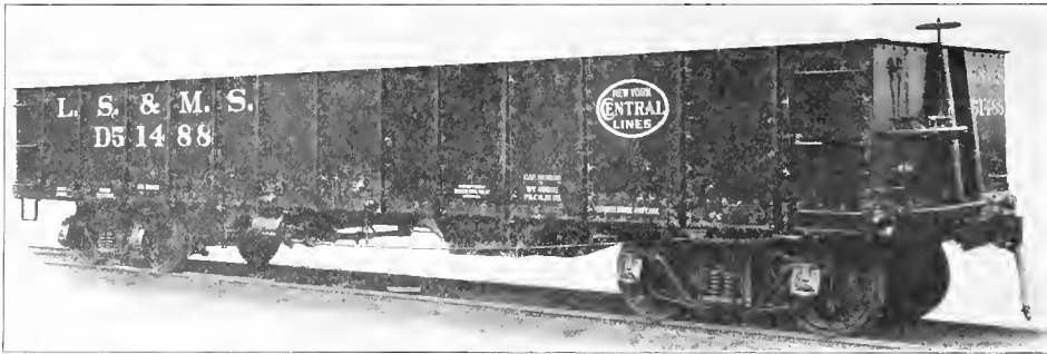
Fig. 41. Gondola Car, Twin Hopper Bottom, Pressed Steel. Capacity, 100,000 lbs. Weight, 40,600 lbs. Pressed Steel Car Co., Builders. (Drawings of this car are shown in Figs. 438-441.)
