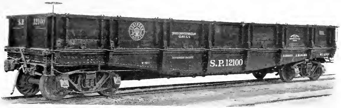
Fig. 88. Hart Convertible Car, Class C. S., Center and Side Dump. Capacity, 100,000 lbs. Weight, 41,800 lbs. Rodger Ballast Car Co., Builders.
