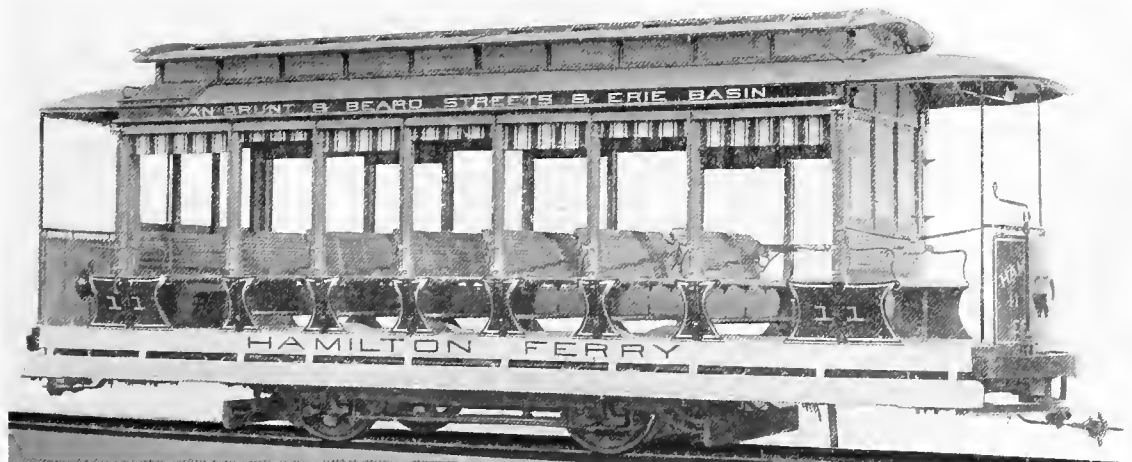
Fig. 6240. Standard 10-Bench Open Car. The J. G. Brill Co., Builders.
