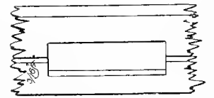
Fig. 2138. Cross-Section of Ridge Pole.
