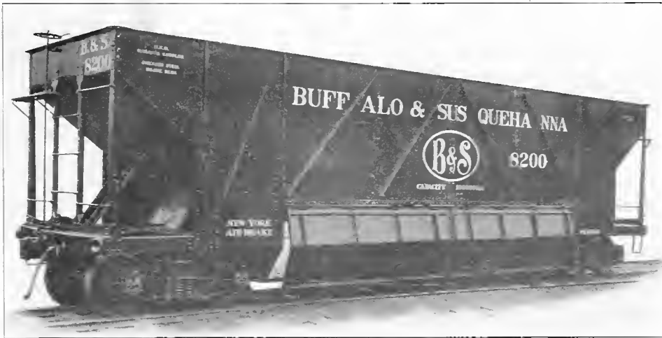
Fig. 75. Coke Car. Pressed Steel. Capacity, 100,000 lbs. Weight, 47,500 lbs. Pressed Steel Car Co., Builders.
