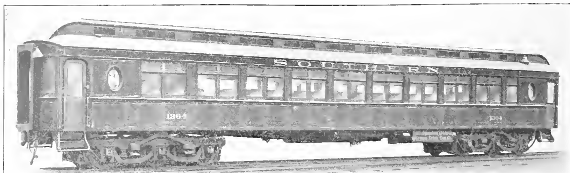
Fig. 136. Steel Vestibuled Coach. Southern. Pressed Steel Car Co., Builders.
