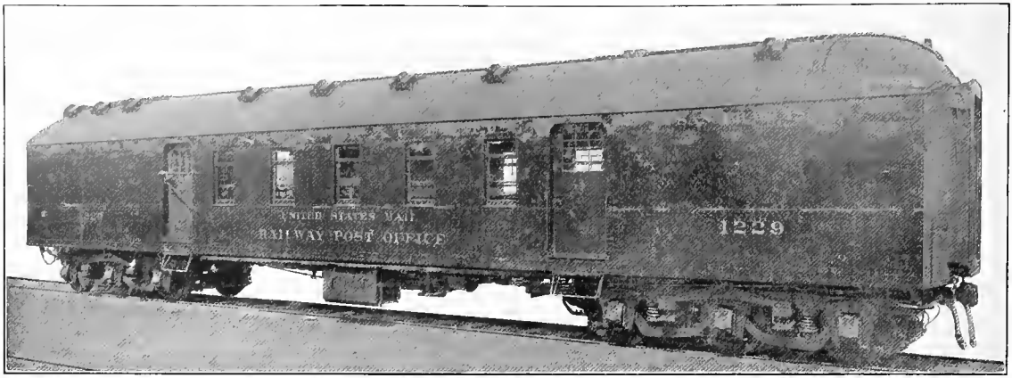
Fig. 194. All Steel Postal Car. Union Pacific. Union Pacific Railroad Co., Builders.
