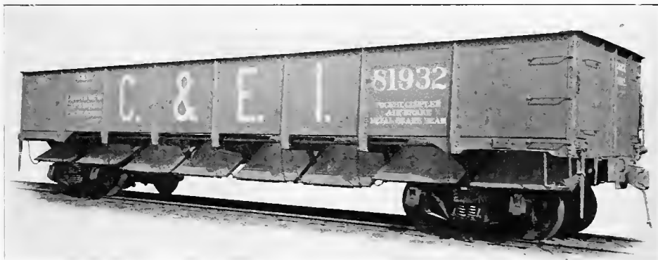
Fig. 82. Dump Car, Drop Bottom, Pressed Steel. Capacity, 100,000 lbs. Weight, 40,500 lbs. Pressed Steel Car Co., Builders.
