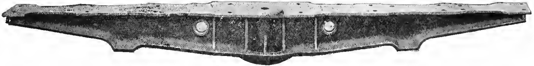
Fig. 1133. I-Shape Cast Steel Body Bolster. American Steel Foundries.
