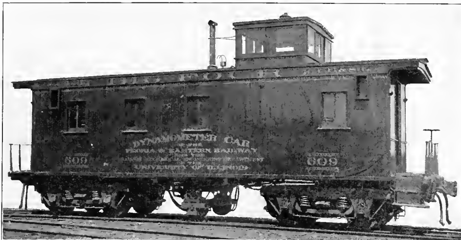
Fig. 261. Dynamometer Car. Big Four. (Drawings of a dynamometer car are shown in Figs. 503-505.)
