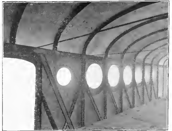
Figs. 1040-1041. Interior Views of Partially Completed All Steel Union Pacific Passenger Coach, No. 499. (Exterior view of this car shown in Fig. 140.)
