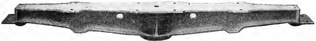
Fig. 1134. Cast Steel Body Bolster. American Steel Foundries.
