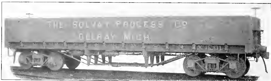
Fig. 43. Wooden Gondola Car with Inside Stakes. Capacity, 80,000 lbs. Middletown Car Co., Builders.
