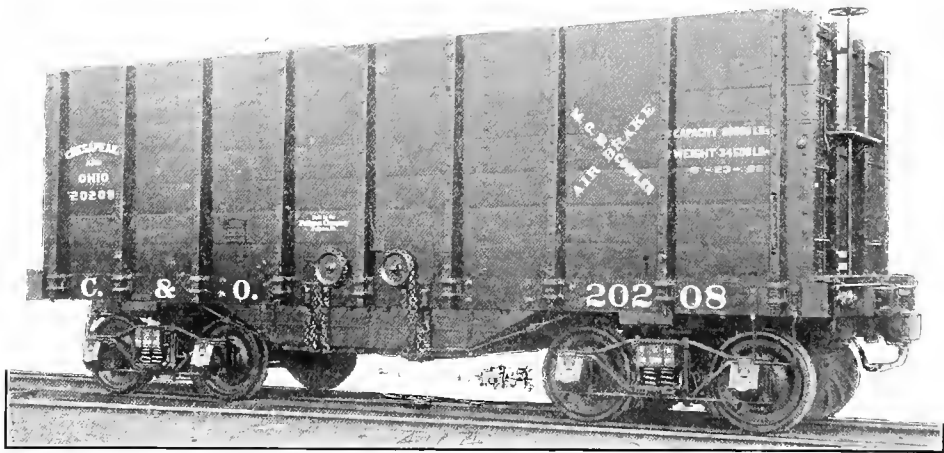
Fig. 57. Coal Car, High Side, Hopper Bottom. Capacity, 80,000 lbs. Weight, 34,500 lbs. Pullman Company, Builders.
