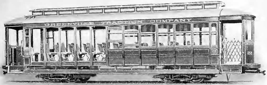
Fig. 6237. Convertible Car. (Both window sashes and metal panels slide into roof pockets.)
