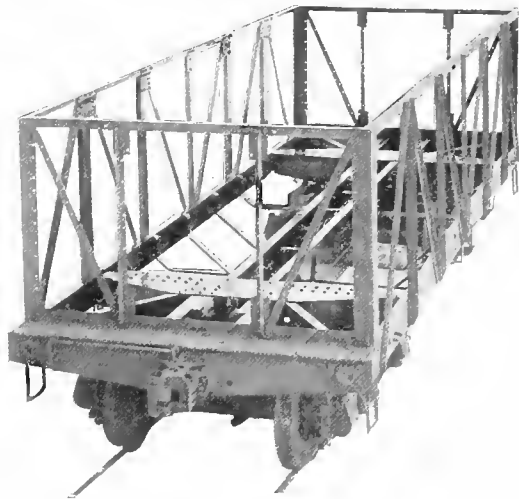
Fig. 1037. Structural Steel Underframe and Side Frame for 80,000 lbs. Capacity Hopper Bottom Gondola Cars. Middletown Car Co.
