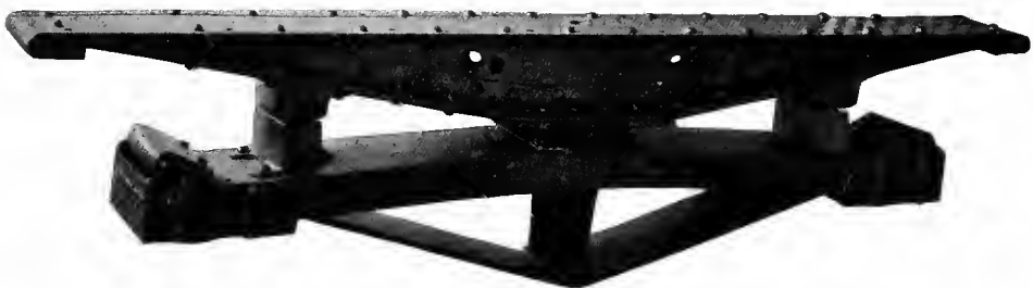
Fig. 1144. Simplex Body and Truck Bolsters with Plate Web Filler. Simplex Railway Appliance Co.
