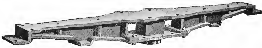
Fig. 1132. Cast Steel Separable Body Bolster for Steel Freight Cars. Commonwealth Steel Co.
