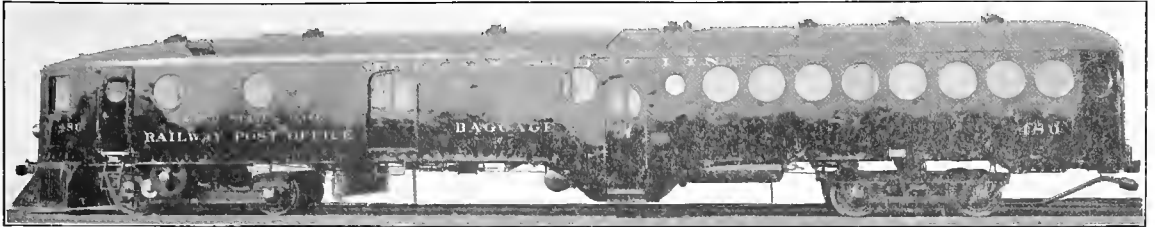
Fig. 206. Gasolene Passenger, Mail and Baggage Motor Car. McKee Motor Car Co., Builders.
