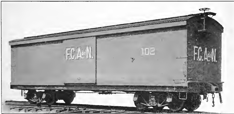
Fig. 9. Box Car, Steel Underframe. Capacity, 66,000 lbs. Weight, 26,400 lbs. Meter Gage. Middletown Car Co., Builders.
