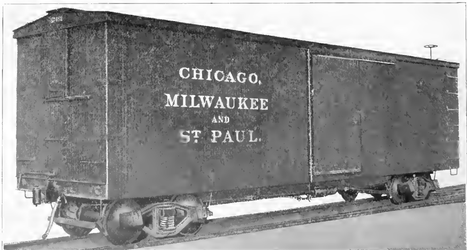
Fig. 7. Box Car, Single I-Beam Center Sill Underframe. Capacity, 80,000 lbs. Weight, 39,300 lbs. Length, 42 ft. Bettendorf Axle Co., Builders.
