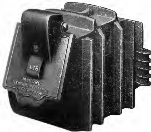
Fig. 5302. McCord Passenger Journal Box with Steel Inserts and Outside Dust Guard.
