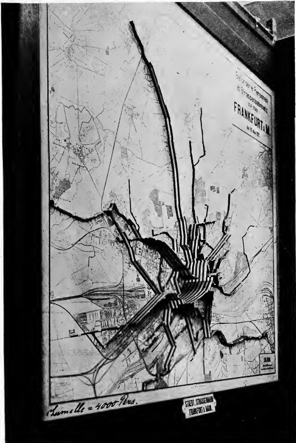
Fig. 185. Passengers Carried in Twenty-four Hours on the Street-car Lines of Frankfurt a M., Germany. Each Vertical Strip Represents 4,000 Passengers The map is about eight feet square. Strips of wood are glued above each street having a car line. This is an excellent presentation of facts
