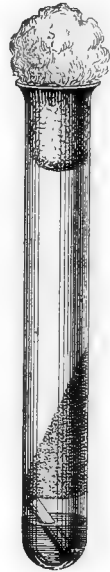
FIG. 209.—Cotton plugged tube with a potato slant resting on a bit of glass rod to keep the potato out of the water in the bottom of the tube. (After Williams, in Schneider, Pharmaceutical Bacteriology , p. 54.)
