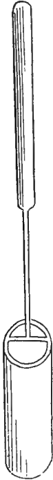
FIG. 210.—Knife punch designed to cut cylinder of potatoes and other vegetables for insertion as slant cylinders in test-tubes as culture media.
