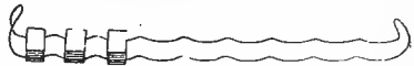
FIG. 46. A simple rack of bent wire suitable for the block-testing outlined in this study.
