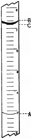
Fig. 15. Diagram of neck of Babcock test bottle; the reading should be made between the points a-b , not a-c .
