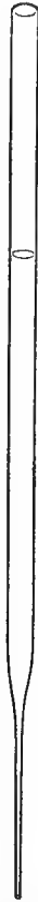
FIG. 30—Capillary pipette. A piece of glass tubing drawn to capillary size at one end. Reduced to three-fourths of the size used. (Original.)
