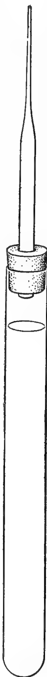
Fig. 31.—Tube in which a suspension of sacbrood larvæ is placed for heating. It consists of a test tube one-half inch in diameter supplied with a perforated stopper through which passes a short piece of glass tubing drawn at one end to capillary size. (Original.)
