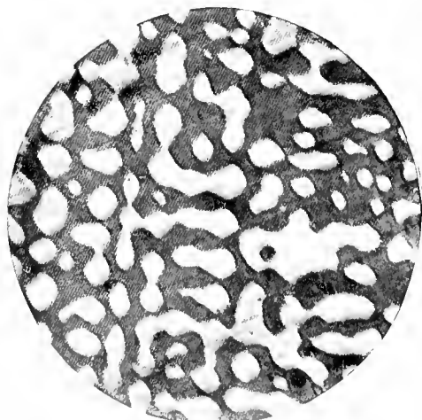
FIG. 5.—Gold-lead alloy lightly etched with 1 per cent. nitric acid. 50 per cent. Pb, 50 per cent. Au. Mag. 140 diams.
