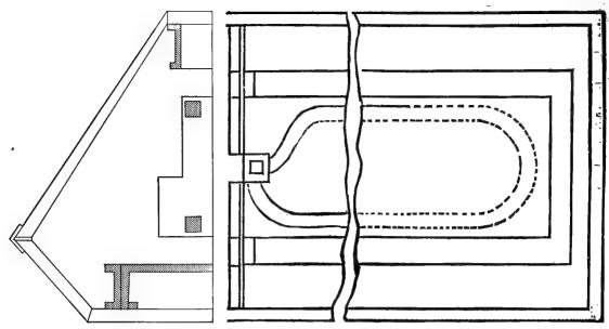
GREENHOUSE, GROUND PLAN AND SECTION, WITH FLUE UNDER CENTRE BENCH.
