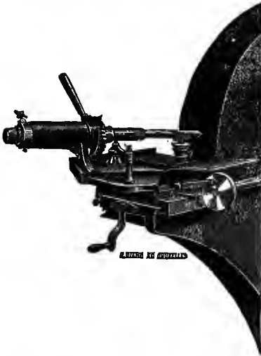
FIG. 8.—Drill grinder; J. M. Demoor, Belgium.
