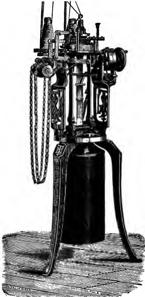
FIG. 33.—The Nye & Tredeick circular rib-cuff machine.
