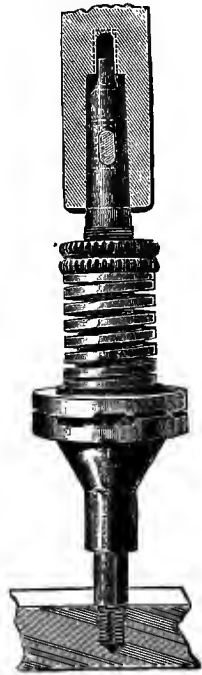
FIG. 15.—Pearn's tapping fixture; exhibited by Smith & Coventry, England.
