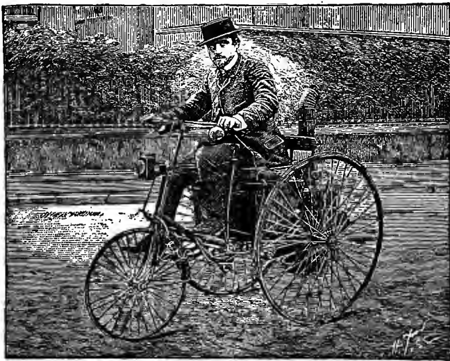
Fig. 17. Serpolet's steam tricycle.
