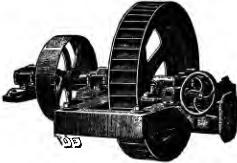
FIG. 73.—General view of vertical Girard turbine, by Brault, Tisset & Gillet.
