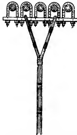
FIG. 178.—Method of attaching the suspension rods.
