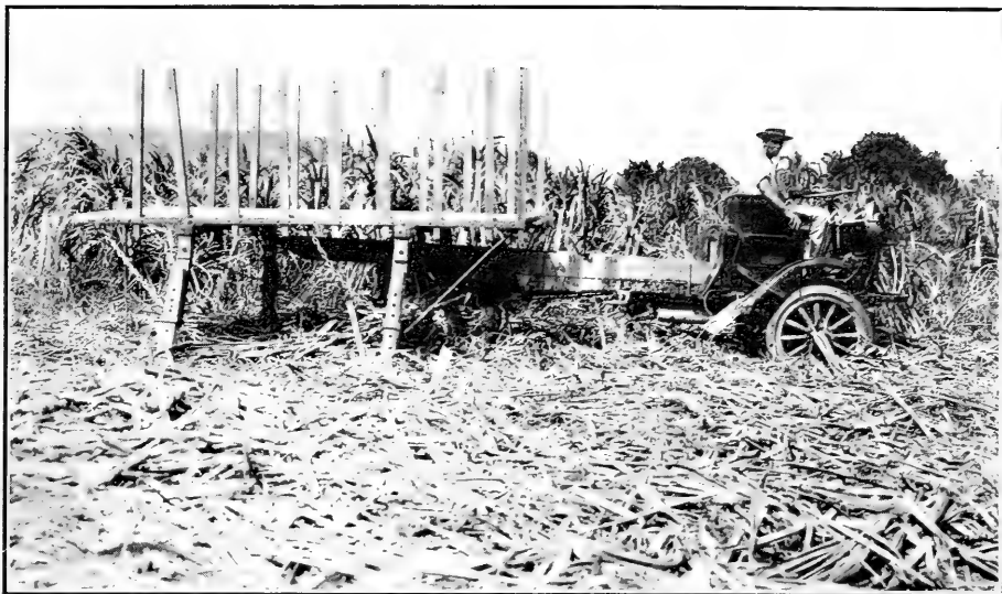
Illustrating How Truck Is Withdrawn From, or Spotted Under, the Thomas Cane Body.
