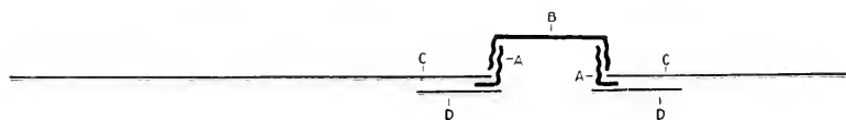
FIG. 57.—Section of tick feeding girdle for experimental purposes. A, threaded and flanged ring; B, cover; C, long adhesive band for girdle; D, short adhesive band covering toothed flange.
