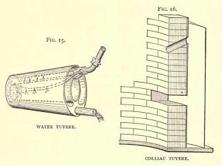
of gas pipe cast inside the tuyere through which water constantly flows. The water tuyere is never used in cupolas when the tuyeres are placed in the sides of the cupola, but it has been used in cupolas in which the tuyere was placed in the bottom and exposed to the heat of molten iron, cinder and slag. When used in this way the tuyere is placed in the centre of the bottom and is made from I to 3 feet long, the mouth being placed at a sufficient height above the sand bottom to
