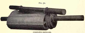
A single casting with Steel Forged Shaft in position. Two such pieces compose the interior working parts of Blowers and Exhausters,
