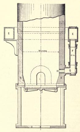
POOR ARRANGEMENT OF BLAST PIPES.
