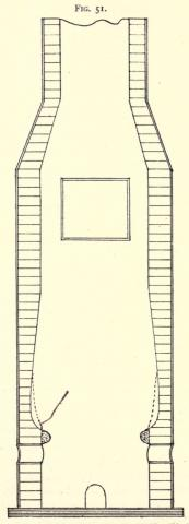
SECTIONAL VIEW LINING OUT OF SHAPE. NO. 2.
