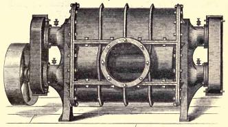
Working parts are two perfectly balanced impellers, mounted on the best steel shafts, running in bronze bushes, detachable journal bearings, cut gearing at both ends of the Blower enclosed in oil-tight casing.
