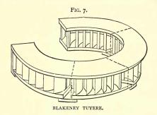
supplied from an outside belt air chamber riveted to the shell. The blast is conducted to the air chamber through one pipe, and, striking the blank spaces sidewise in rear of chamber, passes all around through the curved tuyeres into the centre of the furnace. This tuyere admits the blast freely and evenly to the cupola and very good melting is done with it. All the tuyeres described above may be used with either coal or coke.
