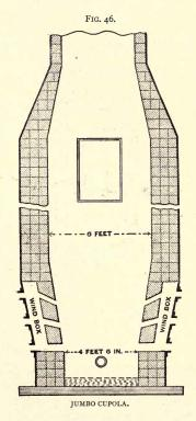
The sprues, gates and foundry scrap are not milled before charging, and the large amount of limestone placed on each charge is required to liquefy the quantity of sand charged into the cupola on the scrap, and prevent clogging and bridging of the cupola. Sixty tons of iron have been melted in this cupola in four hours from the time the blast was put on until the bottom was dropped.
