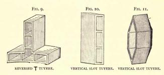
In Figs. 10 and 11 are seen the vertical slot tuyeres used principally in cupolas of small diameter to prevent bridging. They are made from two to three inches wide and ten to twelve inches long, and two or more are placed in a cupola at equal distances apart.
