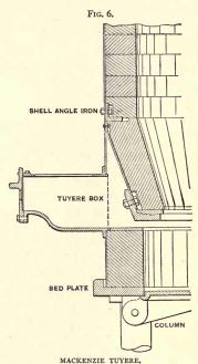
the settling of the stock. The Mackenzie cupolas with this tuyere are constructed of an oval or oblong shape, with an inside belt air chamber. The blast enters the air chamber from a tuyere box at each end of the cupola, and passes into the cupola through a two-inch slot extending all the way round the cupola.
