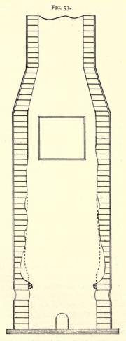
SECTIONAL VIEW OF LINING OUT OF SHAPE. NO. 4.
