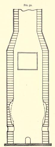
SECTIONAL VIEW LINING OUT OF SHAPE. NO. 3.
