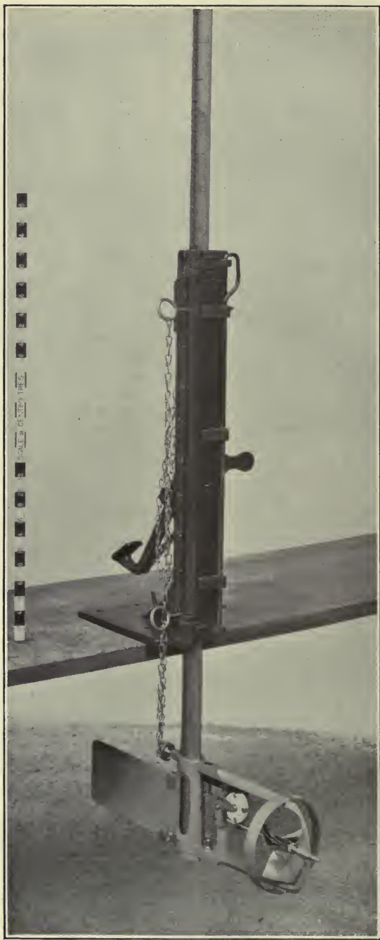
III. STOPPANI CURRENT METER.—Showing meter attached to oval steel rod which is held by the cast iron support.
