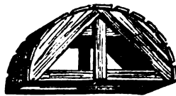
Centering of a Round-headed Arch.
