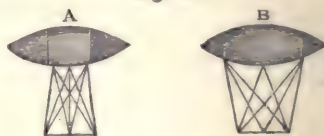
Diagram to illustrate angle of aperture.
