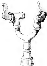
2381. A Y-fixture with Bourcoux brand of nozzle.
