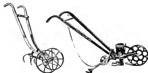
2532. The hand-wheel hoe. 2533. A hand seed-sower.
