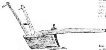
2528. An early Yankee plow, made of wood and the moldboard protected by iron nailed on. After Roberts.
