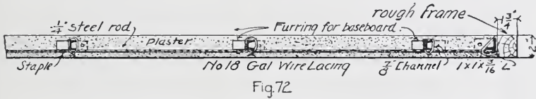
Fig 72 ROEBLING 2IN. WIRE LATH SOLID PARTITION
