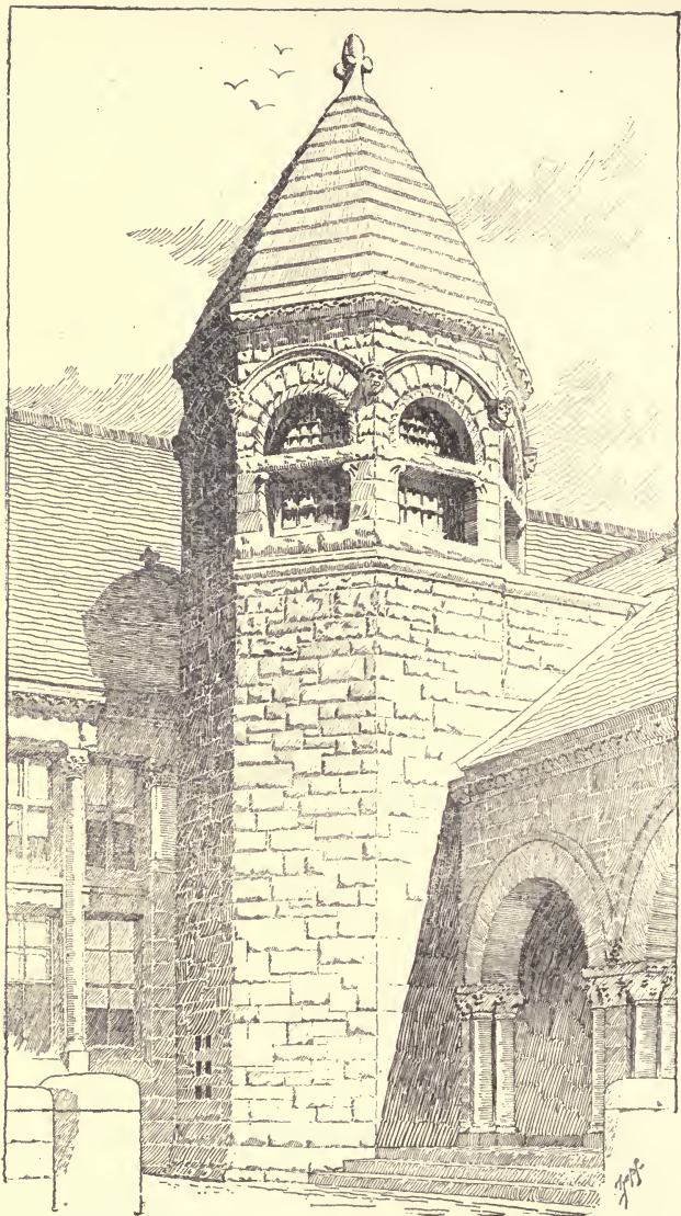
TOWER CONVERSE MEMORIAL LIBRARY, MALDEN, MASS. H. H. Richardson, Architect. Note treatment of shadows in a perspective drawing.
