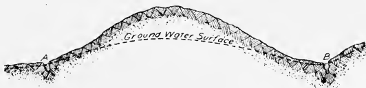
Fig. 2. Relation of Ground Water to Surface Water.
