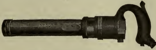
Fig. 58. Pneumatic Riveting Hammer Courtesy Chicago Pneumatic Tool Company
