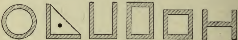
Fig. 155. Typical Cast-Iron Column Sections
