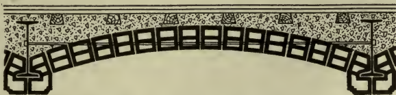
SEGMENTAL TERRA COTTA ARCH CONSTRUCTION
