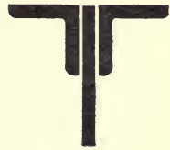
Fig. 4. Chord Section for Heavy Stresses.
