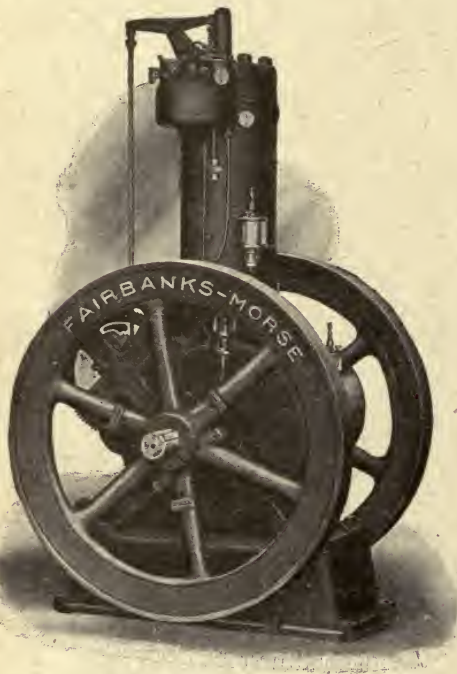
Fig. 134. Typical Single-Cylinder Gasoline Engine for Hoisting Purposes Courtesy of Fairbanks, Morse & Company, Chicago
