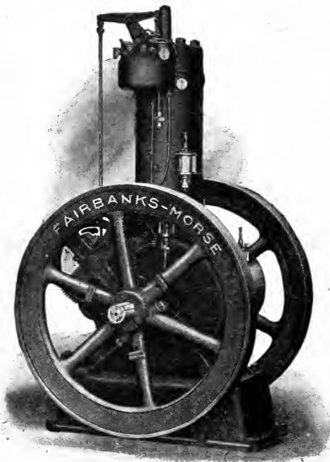
Fig. 134. Typical Single-Cylinder Gasoline Engine for Hoisting Purposes Courtesy of Fairbanks, Morse & Company, Chicago
