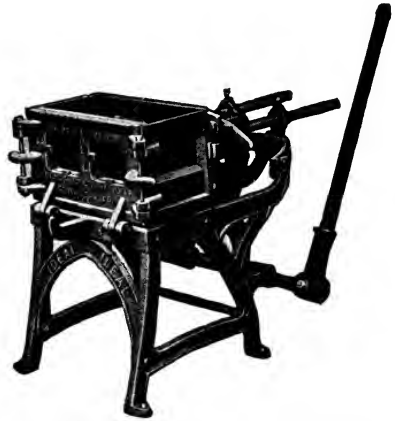
Fig. 152. "Ideal" Concrete Block Machine Courtesy Ideal Concrete Machinery Company, Cincinnati, Ohio
