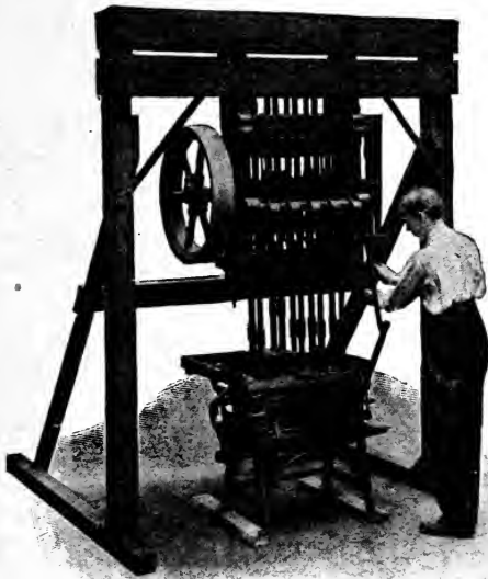
Fig. 153. "Ideal" Automatic Tamper Used in Connection with Block Machine Courtesy of Ideal Concrete Machinery Company, Cincinnati, Ohio
