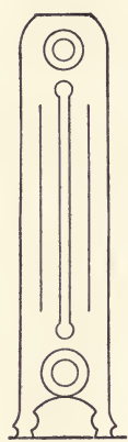
Fig. 87. End Elevation of Radiator Showing Taps at Top and Bottom for Pipe Connections.
