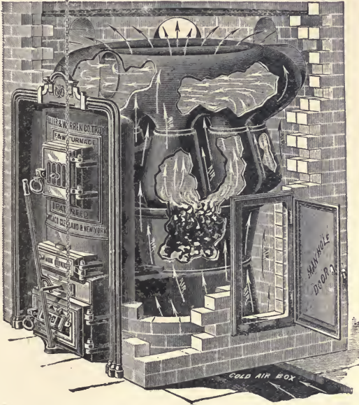
Fig. 6. A Common Type of Direct-Draft Furnace in Brick Setting. Cast-Iron Radiator at Top.
