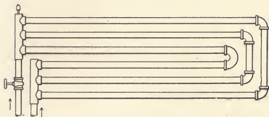
Fig. 98. Circulation Coil, One Method of Construction. Supply Pipes may be Either Drops or Risers.
