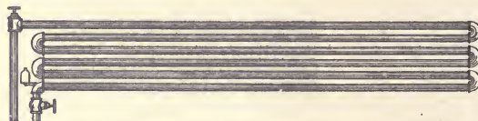
Fig. 21. "Trombone" Coil. Used where Entire Coil must be Placed on One Side of Room
