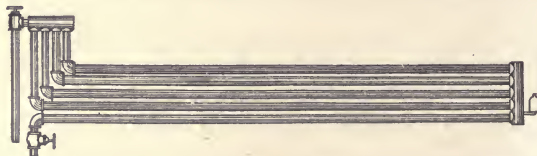
Fig. 22. "Miter" Coil. Adapted, like the "Trombone," Only to a Single Wall. Frequently Used in Factories and Shops.
