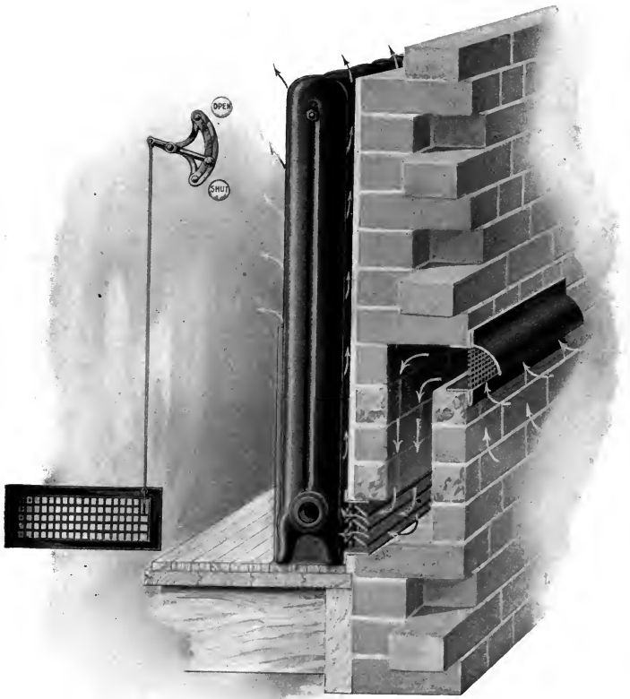
DIRECT-INDIRECT SYSTEM OF WARMING, SHOWING ADJUSTABLE DAMPER. American Radiator Company.
