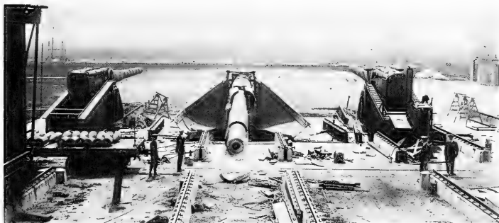
Inspection of a 14"/45 MARK II-1 gun that exploded after the second round was fired, May 1924.
