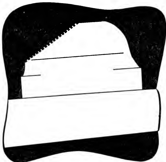
ENLARGEMENT OF FIXED SIGHTS SHOWING INEXPENSIVE METHOD OF CORRECTING LIGHT REFLECTION WHICH IMPAIRS SIGHTING.
