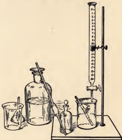
FIG. 13.—Apparatus for testing acidity of milk.
