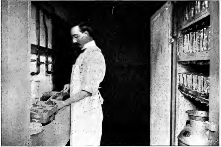
CUT 41. MILK BOTTLES AND DAIRY UTENSILS ARE WASHED AND RINSED IN SINK ON LEFT, THEN PLACED IN BRICK STERILIZER ON RIGHT, DOOR CLOSED AND LIVE STEAM TURNED IN FOR 20 MINUTES.
