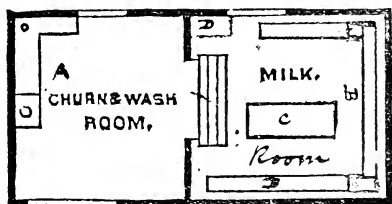
Fig. 38.—GROUND PLAN OF MILK-HOUSES (Figs. 36 and 37).
