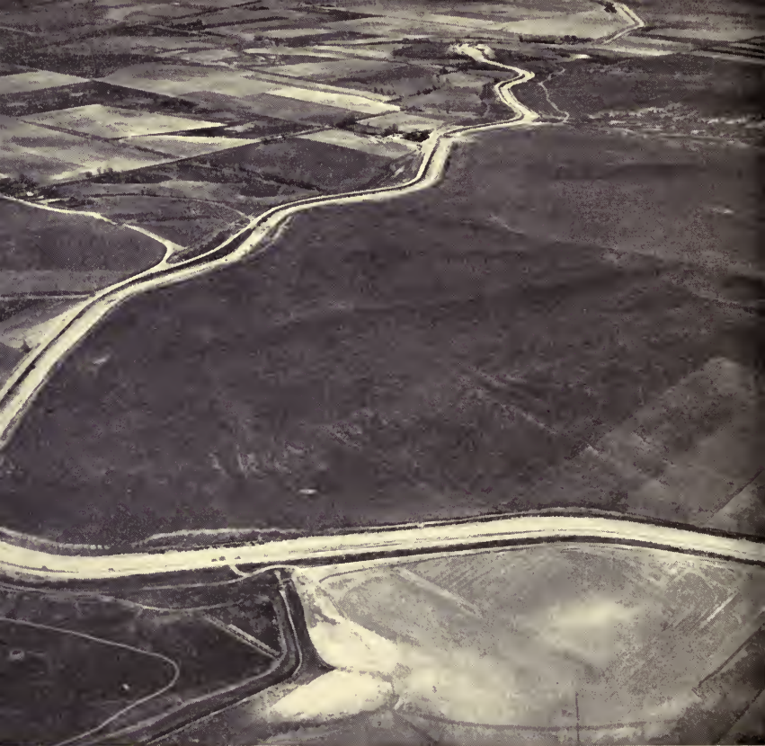
6. How irrigation works. The broad ditch, winding down a natural grade, feeds lateral ditches that serve farm fields. The high ground at right center is dry. BUREAU OF RECLAMATION.
