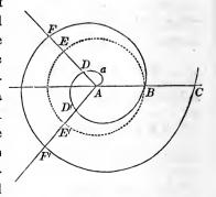
have moved along it to some point as D, and will have described the arc AaD of the spiral. When the line takes the position AD'E' the point will have described the curve AaDD', and when the line shall have completed an entire revolution the point will have described the curve AaDD'B.
