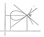
the curve, until x=a when they unite at the point M. For x>a there will be two real values of y and consequently two branches of the curve. The point M, at which the branches intersect each other, is called a *multiple point*, and differs from a cusp by being a point of intersection instead of a point of tangency. At the multiple point M there are two tangents, one to each branch of the curve. The one makes an angle with the axis of abscissas, whose tangent is
