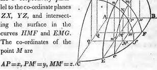
It is now evident that the solid whose base on the co-ordinate plane YX is the rectangle AQM'P, may be extended indefinitely in the direction of the axis of X without changing the value of y, or indefinitely in the direction of Y without changing x. Hence, x and y may be regarded as independent variables.
