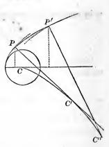
and hence, the difference between the radii of curvature at any two points of the involute is equal to the part of the evolute curve intercepted between them.
