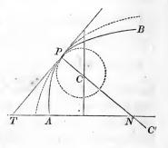
also apparent, that the centre may be taken at some point C', so remote from P, that the circumference shall fall between the curve APB and the tangent PT, and then every circumference described with a greater radius will fall without the curve. Hence, there are two classes of tangent circles which may be described; the one lying within the curve, and the other without it.
