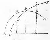
for h negative: hence, the two lines qs, q's', have contrary signs. The curve, therefore, lies above the osculatory circle on one side of the point P, and below it on the other, and consequently, divides the osculatory circle at the point of osculation. Hence, also, the osculatory circle separates the tangent circles which lie without the curve from those which lie within it (Art. 151).
